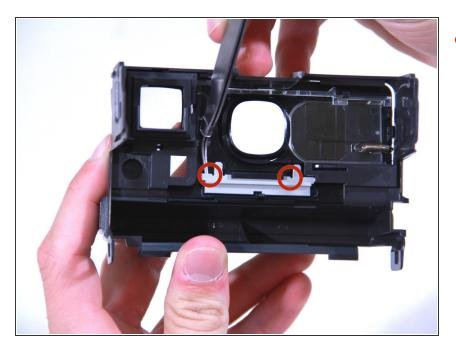
Pry off the slider (the light gray piece) by slipping it out from beneath the tabs (their location is indicated by the two red circles).
