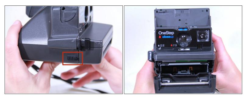
• Slide the action button, on the bottom of the camera, to open the bottom.
