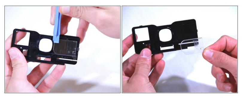
Make sure the last plastic piece is set all the way to the right. Using the blue plastic tool, pry it loose. It should easily pop out.
