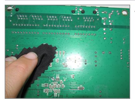
Turn the motherboard on its back side and completely wipe away any small particles.
