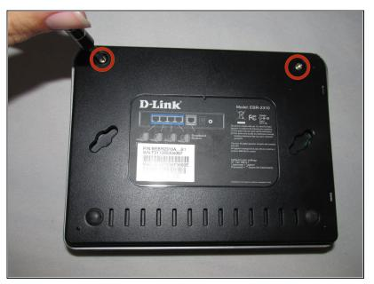
• Using a Phillips #2 screwdriver, remove the two top screws.
