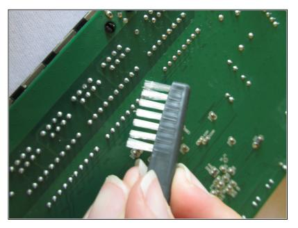
Using the same toothbrush, brush the tiny crevices on the back side of the motherboard.
