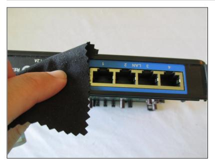
Wipe the cable connector compartments using the same soft cloth.
