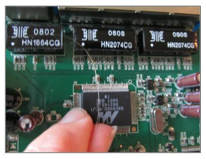
Once you have completely removed your logic board from its casing, look for any large dust particles and/or other dirt inside the router. Gently remove these particles with your fingers.
