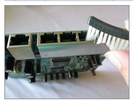
Using a soft bristle toothbrush, brush the insides of the cable connectors in order to remove any hard-to-reach dust.
