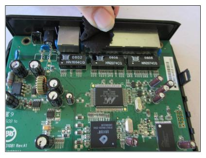
Using your cloth, gently wipe the metal slates around the cable connectors.
