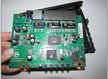
• Use a Phillips #2 screwdriver to remove the two screws at the bottom of the motherboard.
