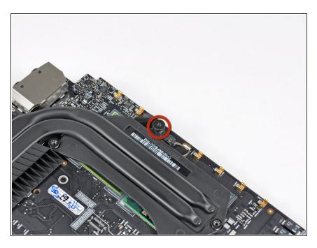
Remove the single 5 mm T6 Torx standoff from the heat sink.
