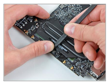
To disconnect the heat sink thermal sensor, pinch its cables between your thumb and a spudger and pry the spudger upward to lift the connector up and out of its socket on the logic board.
