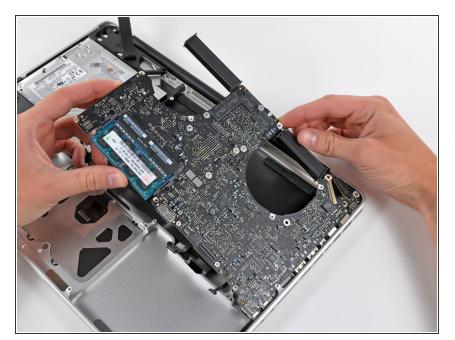
Carefully lift the logic board assembly from the left side and work it out of the upper case, minding the
