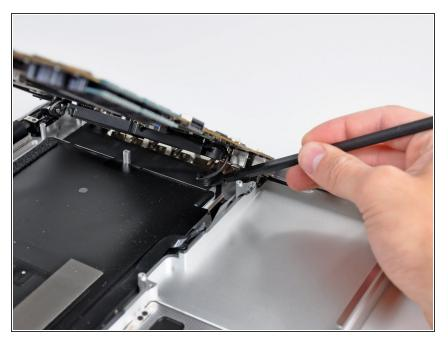
• Lift the logic board enough to gain clearance and use a spudger to pry the microphone up off the upper case.
