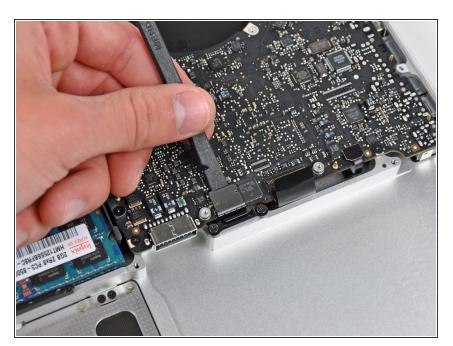
Use the flat end of a spudger to pry the trackpad cable connector up out of its socket on the logic board.
