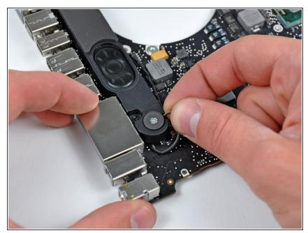
(i) If necessary, lift the microphone out of its recess in the left speaker housing.
