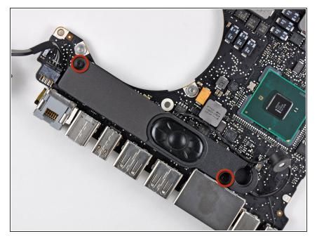
Remove the two 5 mm Phillips screws securing the left speaker to the logic board.
