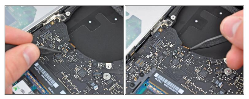
• Use the tip of a spudger or your fingernail to flip up the retaining flap on the keyboard backlight ribbon cable socket.
