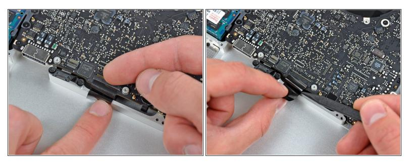
• Use your fingernail to carefully flip up the keyboard ribbon cable retaining flap.
