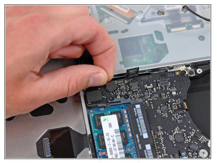
• Carefully pull the subwoofer/right speaker cable up to lift its connector out of its socket on the logic board.
