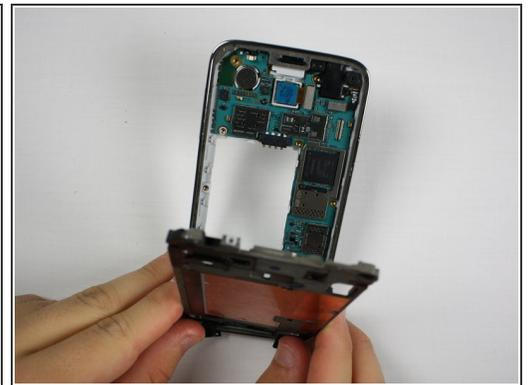
**⚠ Spread pressure out evenly to avoid damage or bending of the midframe.**
