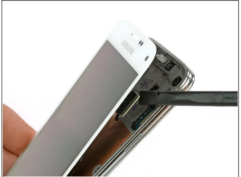
**⚠** Keep the top portion of the display assembly next to the frame.
