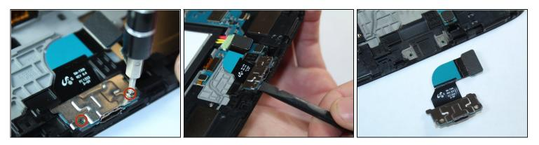
• Unscrew the 2.9mm screws from the charging port with Phillips Head #000 and use the spudger to pry it up from under the port to remove component from the device.
