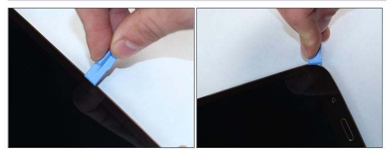
• Start out by separating the screen from the back cover using the larger plastic opening tool to pry them apart.
