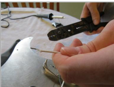
Use wire cutters to strip about 1/2" of shielding off the wire.
