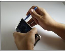
Gently remove the volume button. Using a plastic opening tool or guitar pick, loosen the back panel of the phone. Work around the phone, following the crease of the back panel.
