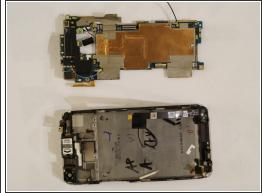
Completely remove the motherboard.
