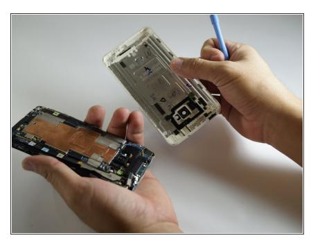
Pry the back loose and lift. The back panel will come off with time.
