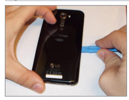
Using the plastic opening tool, or the thin side of the spudger to separate the back cover from the phone. Start at the bottom corner of the phone. Be gentle because it may cause cosmetic and internal damage if not done with care.
