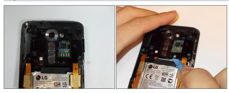
• After all visible screws have been removed use the spudger to pop off the top plastic cover.
