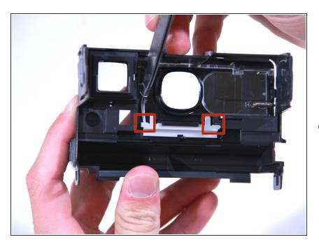
Once you have the face plate removed the first thing to do is pry off the slider (the light grey bar near the bottom). The easiest way to
