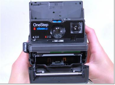
Slide the action button, on the bottom of the camera, to open the bottom.
