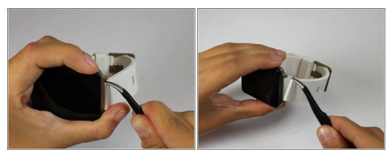
A This is a challenging step. Do it carefully to prevent the spring bar from flying out of the wristband.
