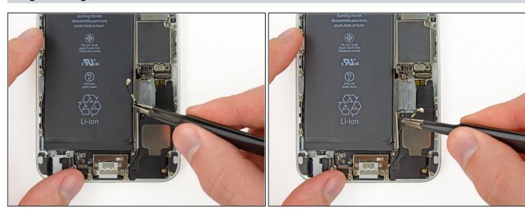
• Grasp the antenna connector with a pair of tweezers and carefully begin de-routing it from its channel on the speaker.
