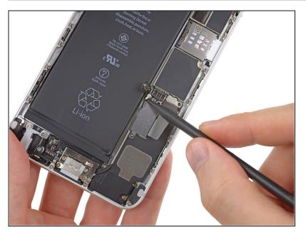
Use the tip of a spudger to disconnect the interconnect antenna cable from its socket on the logic board.
