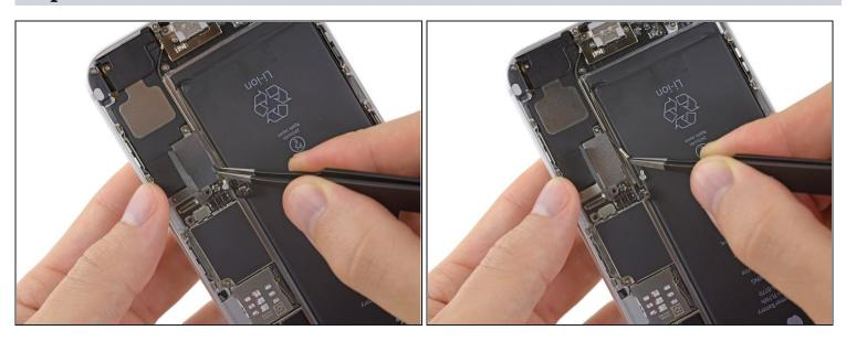
• Grasp the interconnect antenna cable with a pair of tweezers and carefully de-route it from its channel on the vibrator assembly.
