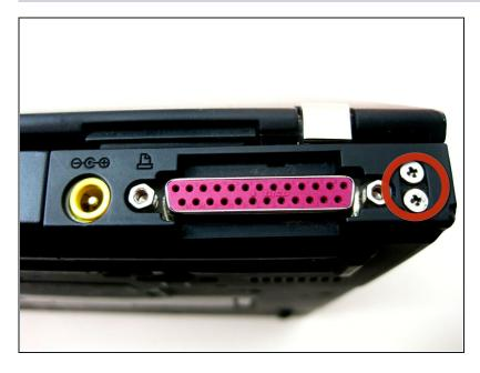
Unscrew the four Phillips screws located on either side of the rear of the T42 (there are two located on each end.)
