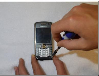
Turn the phone over so that the screen is facing up. With the bottom cover off, you will be able to locate two 7.5mm Torx #T6 screws in each corner below the keyboard. Carefully remove these.
