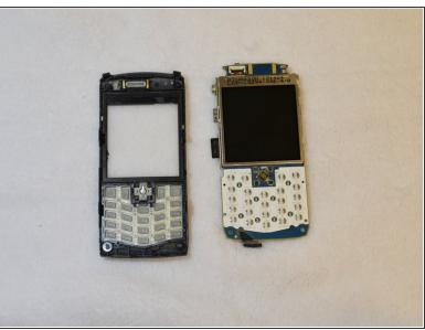
• The front panel is now ready to be removed from the rest of the phone. To do this, just pry the front part (with the keyboard and screen) away from the logic board of the phone with your fingers.
