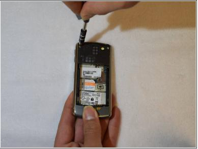
Now that the battery cover has been removed, locate the two 7.5mm Torx #T6 screws at the top of the phone. Remove these by turning counter-clockwise with your T6 screwdriver.
