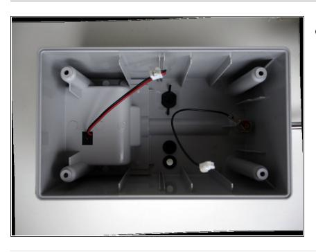
Back cover interior view with both battery and antenna cable.
