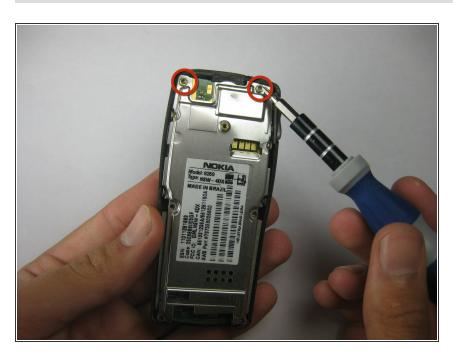
Remove the two screws at the top.
