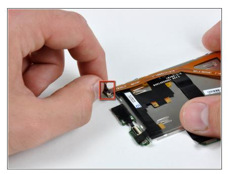
• Peel away the black tape to reveal the display data cable connector.
