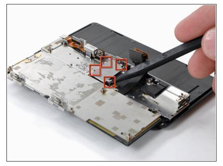
• Remove the EMI shield by releasing the clips shown with the tip of a spudger.
