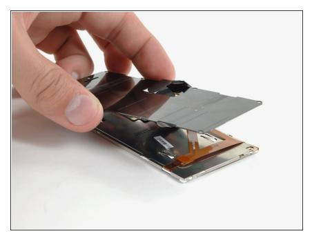
• Lift the back cover off the display assembly, feeding the ribbon cable through the slit as you go.
