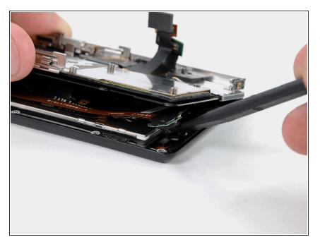
Use the flat end of a spudger to lift the board that contains the ambient light sensor and display data cable connector out of the screen housing.
