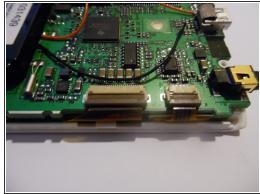
Using tweezers, or something similar flip up the tab, releasing the wires located under the flap.
