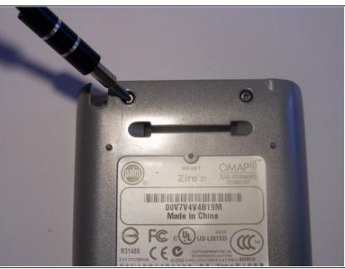
Remove the two 0.8mm screws located on the back of the device.
