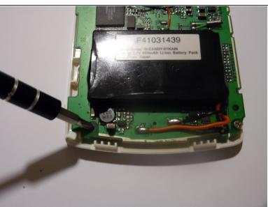
Using a Philips head screwdriver, remove the two screws located at the bottom of the board.
