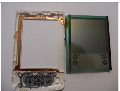
Carefully, remove the screen from the device by lifting up and replacing with a new one.
