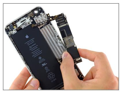
• Lift and remove the logic board out of the iPhone.
