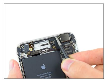
Use a pair of tweezers to peel back the piece of tape covering the hidden screw securing the rear-facing camera bracket to the rear case.
