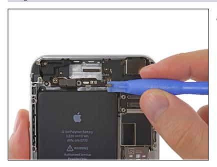
Carefully pry the 5GHz Wi-Fi antenna connector up off the logic board with a plastic opening tool.
