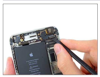
Use the flat end of a spudger to disconnect the rear-facing camera connector from its socket on the logic board.
