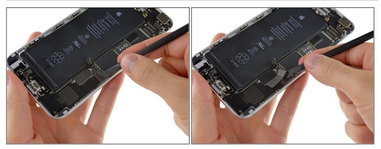
• Pry the charge port connector cable up from its socket on the logic board with the flat end of a spudger.
