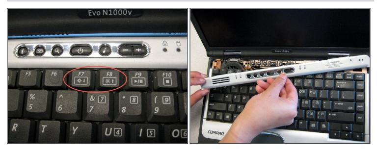
• Insert a spudger between the *F7* and *F8* keys. Lift up to remove the LED cover.
