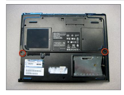
Remove the two TM 2.5mm x 8.0mm screws that secure the top cover to the base.
