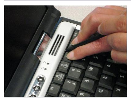
While holding the Scroll and Pause keys, insert a spudger between the keys into the notch in the LED cover. Lift up.
