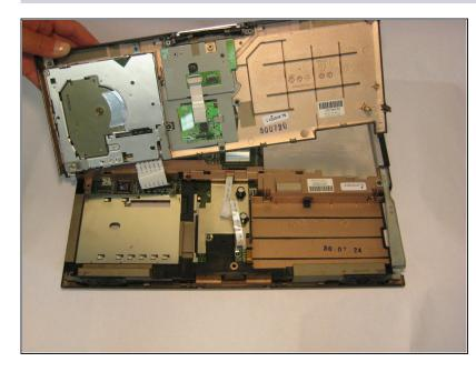
• Lift the the palm rest up from the front edge of the laptop and swing it towards the screen.
