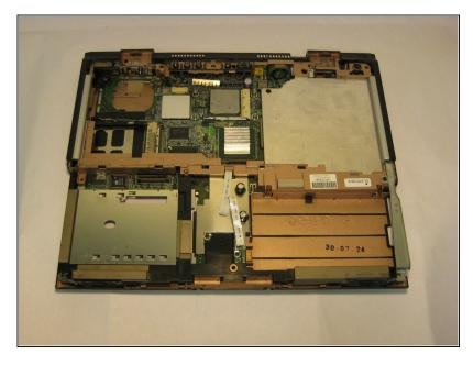
• Turn the base top side up with the front facing forward.
