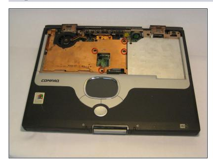
• Remove the four screws from the heat sink.
