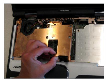
• Pull the the heat sink up and out of the computer.
