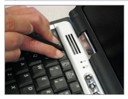
• While holding the **F1** and **F2** keys, insert a spudger between the keys into the notch in the LED cover. Lift up.
