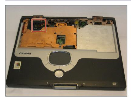
• Disconnect the cable connecting the fan to the system board.
