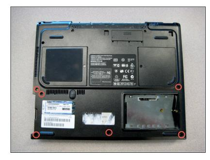
• Using the TR8 Torx screwdriver, remove the six screws from the back case.
