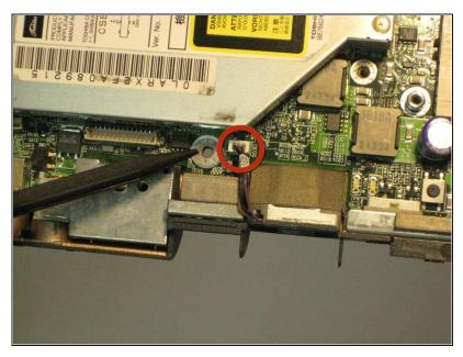
• Disconnect the fan cable from the system board.
