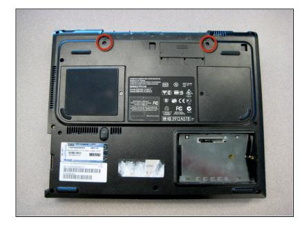
• Using a TR8 Torx screwdriver, remove the two T8 Torx screws that secure the LED cover to the base enclosure.
