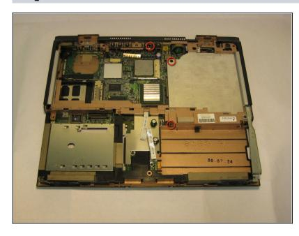
Remove the three TM 2.5 mm x 5.0 mm screws that secure the top cover to the base.
