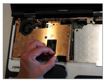
• Pull the the heat sink up and out of the computer.
