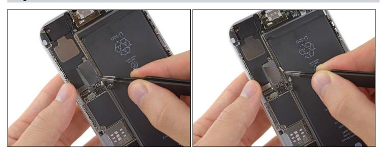
• Grasp the interconnect antenna cable with a pair of <u>tweezers</u> and carefully de-route it from its channel on the vibrator assembly.
