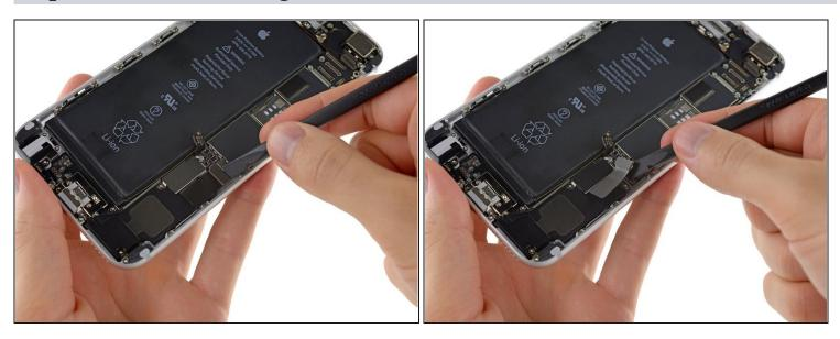
• Pry the charge port connector cable up from its socket on the logic board with the flat end of a spudger.
