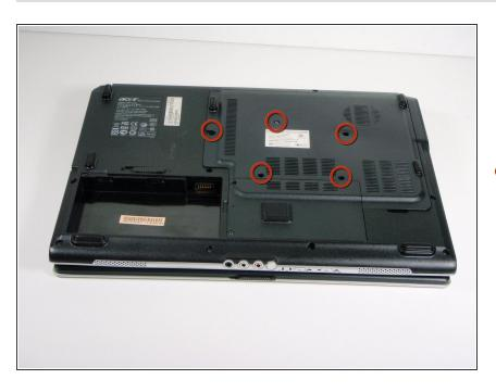
Locate and remove the 5 screws that secure the panel over the RAM and CPU cover on the upper right
