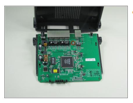
Remove one small Philips screw from the logic board so you can remove the bottom panel.
