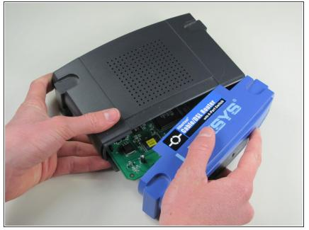
(i) There actually aren't any screws or notches under the rubber feet on this model. A little force is all that's needed to pull off the front blue panel. (The front is held on by a recess/notch on each side)
