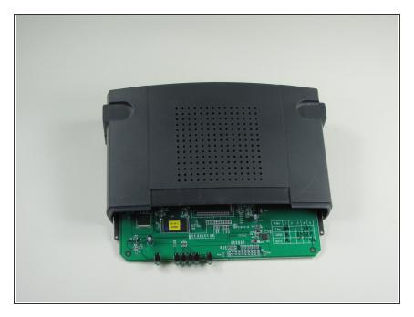
Once the front blue panel is off, the top panel slides back and then comes off easily (it's connected to the bottom panel by two plastic notches).
