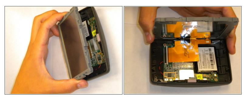
• Lifting from the upper edge of the screen, tilt the screen away from the device.
