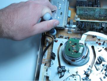
With the device front facing you remove the six screws with a phillips head screwdriver around the VHS drive.
