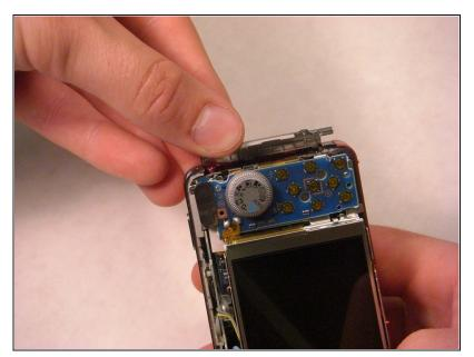
After removing the screws, gently pop open the plastic piece, as shown by firmly pulling it with your fingers.
