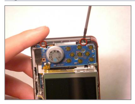
Remove the two screws at the top of the camera casing.
