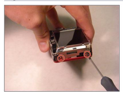
Remove the two screws connecting the front casing to the electrical components using a screwdriver.
