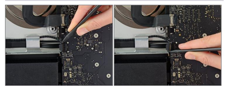
• Push on each side of the left speaker cable connector with the tip of a spudger and gently *walk* it out of its socket.
