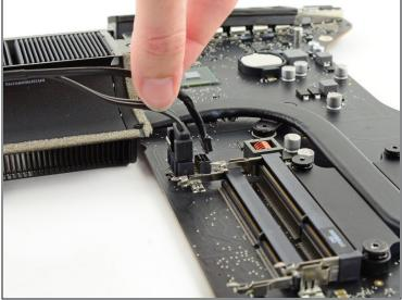
Grasp the hard drive power connector and gently pull it out of its socket on the logic board.
