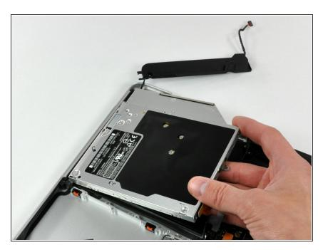
Lift the optical drive from its right edge and pull it out of the computer.
