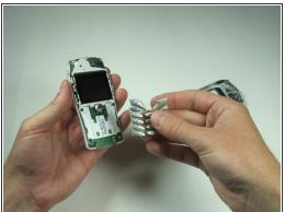
After removing the screws, the two halves will separate. If not, then pry them gently apart.
