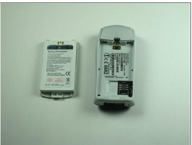
Remove the battery from the back.
