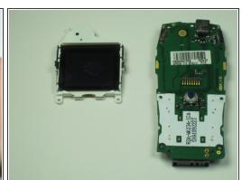
Carefully remove the plastic clips holding the screen on the board.
