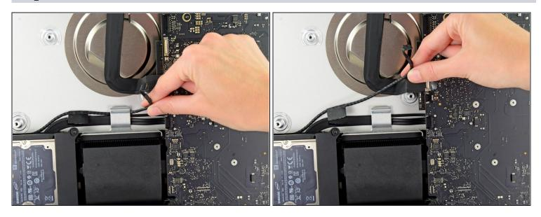
• Gently lift the left speaker cable upwards to de-route it from the clip holding it to the rear case.
