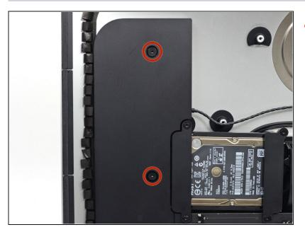
Remove the two 10.0 mm T10 screws securing the left speaker to the rear case.
