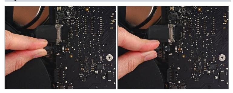
• Pull the fan cable connector straight away from its socket on the logic board.
