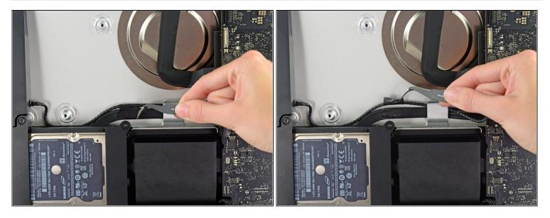
(i) If necessary, use a pair of tweezers to peel the tape securing the left speaker cable to the SATA data/power cable.
