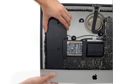
• Lift, but do **not** remove, the left speaker straight up, until the power button cable is exposed (about 0.5").
