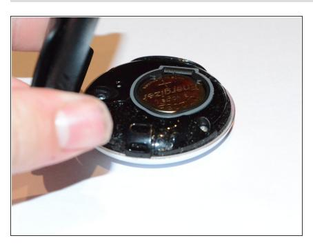
Remove the Rear Cover from the Device
