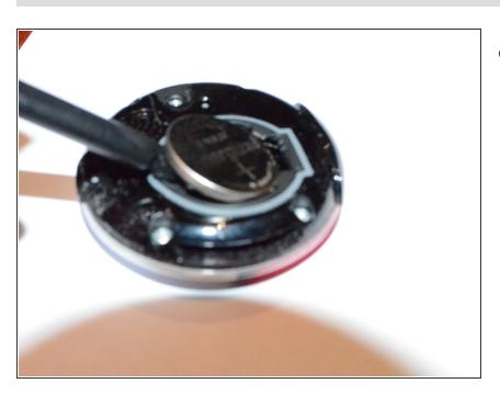
Use the flat end of a Spudger to Remove the Battery
