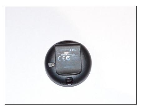
Locate the Screw on the Back of the Pokewalker.
