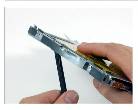
Use a spudger to carefully pry the silver metal bracket off the left side of the optical drive. Be careful not to bend the bracket, as it is very thin and bends easily. If the bracket doesn't come free easily, heating the adhesive may make prying the bracket off easier.
