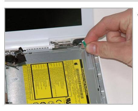
Lift the Bluetooth antenna board from the right side of the optical drive.
