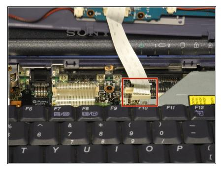
Put the speaker panel's ribbon cable back in place.
