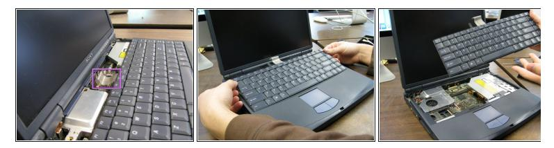
To remove the keyboard, lift it a few inches from the computer, taking care not to pull beyond the length of the ribbon cable that secures it to the motherboard.
