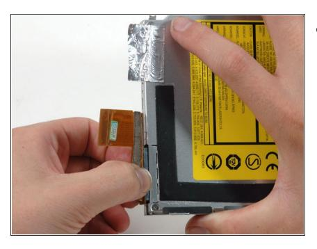
Disconnect the orange cable from the optical drive.
