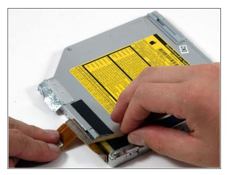
Peel up the orange tape partially covering the orange optical drive cable.
