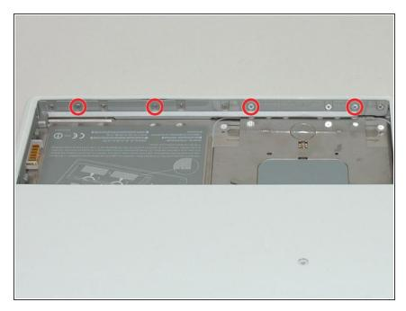
Remove the four 3 mm indicated Phillips #00 screws from the front wall of the battery compartment.
