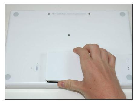
• Lift the battery out of the computer.
