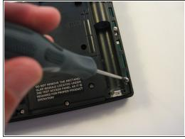
Using a Philips Screwdriver #00 unscrew the twelve 11.8mm screws shown in the picture and located on the back of the calculator.
