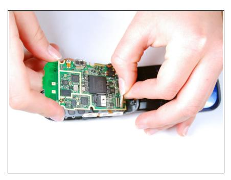
Remove the pin socket that connects the screen to the motherboard by pulling up away from the motherboard.
