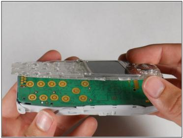
• Insert spudger between screen assembly and phone body.
