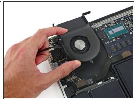
Lift the end of the fan closest to the display hinge and remove the fan from the upper case.
