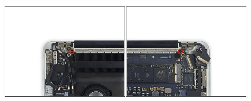
Remove the two 4.2 mm T5 Torx screws securing the aluminum hinge brackets (one on each side of the Macbook).
