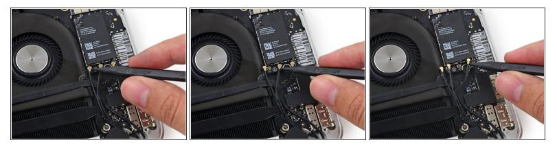
Insert the tip of a spudger under each of the antenna cables near their connectors and pry up to disconnect them from the AirPort board.
