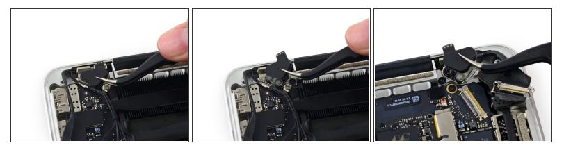
• Remove the rubber hinge covers from the right and left display hinges.
