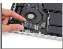
Lift the free end of the AirPort board up slightly and pull it straight out of its socket on the logic board.
