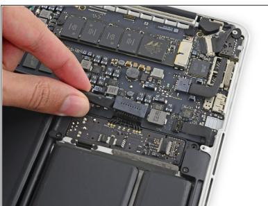
Use the flat end of a spudger to lift the battery connector straight up out of its socket on the logic board.
