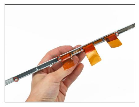
Remove the five small Phillips screws securing the plastic antenna cover to the inside of the clutch cover.
