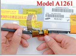
Carefully lift the inverter out of the clutch cover.
