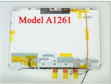
Remove the two pieces of tape securing the display data cable to the LCD.
