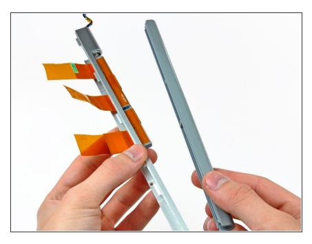
Pull the antenna cover off the clutch cover, being careful not to damage the antenna cables.
