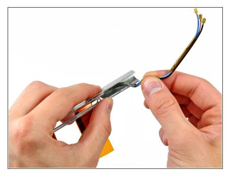
If necessary, peel the antenna leads off the adhesive securing them to the clutch cover.
