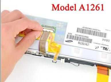
• Disconnect the display data cable from the LCD by pulling it toward the bottom edge of the display.
