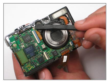
• Lift up the metallic-colored clip with the spudger to remove the shutter panel.
