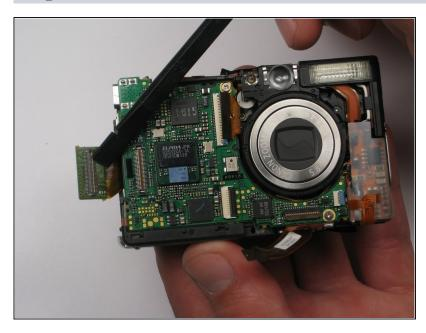
• Pull the flap back with the spudger so that the logic board is exposed.
