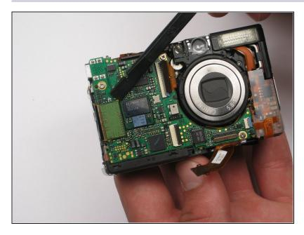
• Lift up the large green flap by using the spudger to pry up top right yellow edge.
