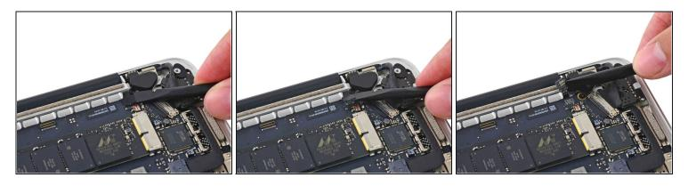
• Use the flat end of a spudger to disconnect the keyboard backlight cable and bend it up out of the way of the logic board.
