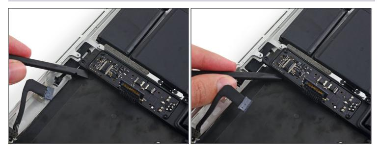
• Use the flat end of a spudger to wedge the battery contact board up slightly to allow room to extract the dual microphone assembly.
