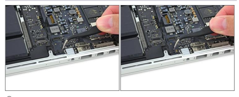
$\widehat{\boldsymbol{\imath}}$  If necessary, peel back any tape covering the microphone cable ZIF connector.
