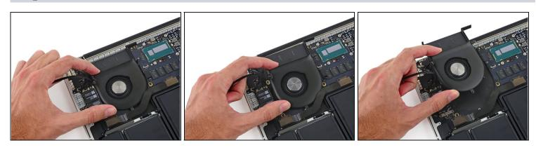
• Lift the end of the fan closest to the display hinge and remove the fan from the upper case.
