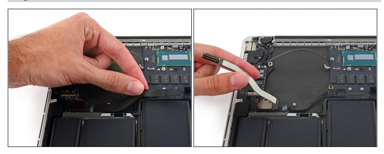
• Lift the logic board end of the I/O board cable straight up to bend it out of the way.
