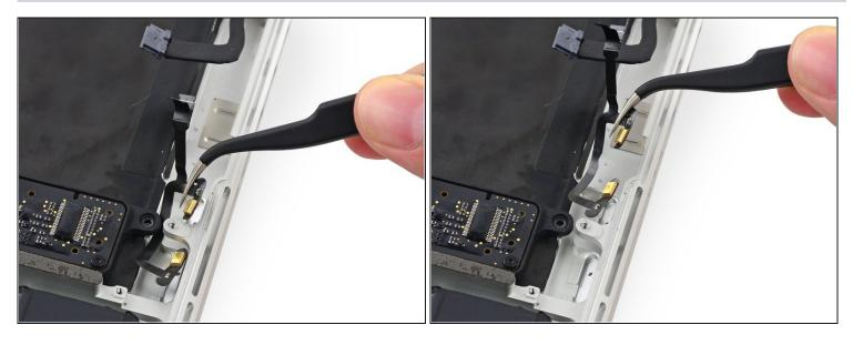
• Pull the dual microphone cable assembly up and toward the logic board recess to remove it from the upper case.
