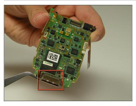
Replace logic board to replace charging adapter.
