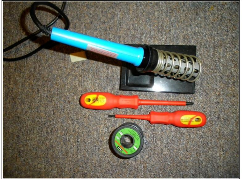
**i** I used 1000v insulated electricians screwdrivers, as I like to be safe when working on electronics that have a higher risk of zapping me.
