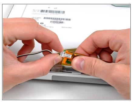
• Disconnect the backlight cable from the inverter board.
