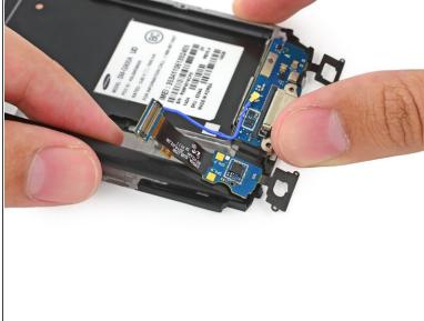
Gently slide the flat end of a spudger in between the daughterboard cable and the interior midframe to begin to separate the adhesive holding it down.
