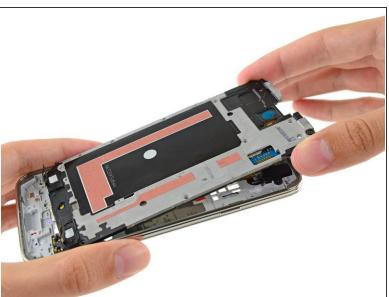
• Carefully remove the interior midframe/motherboard assembly from the white inner midframe.
