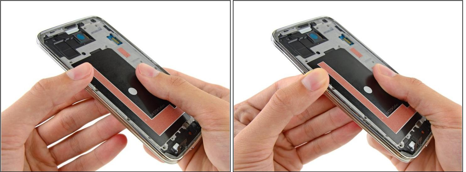
ⓘ The midframe is composed of two halves that encase the motherboard.
