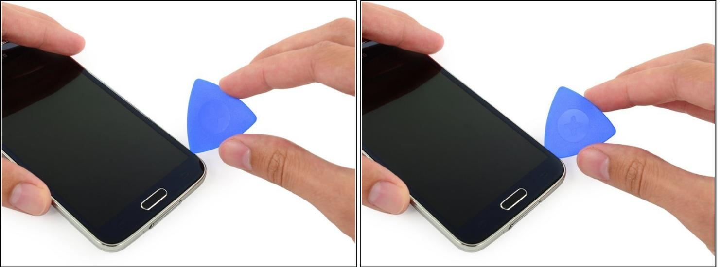
ⓘ In the following steps you will be using an opening pick to separate the adhesive securing the front panel glass. Only pry where directed. If you experience resistance, stop sliding the opening pick and reapply heat.
