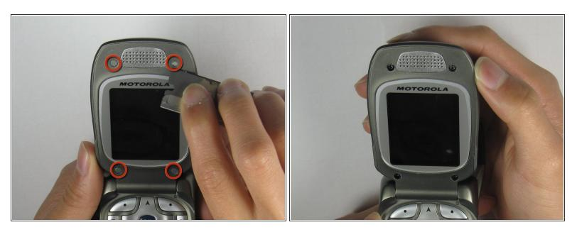
Use a Razor Blade to remove the screw covers.
