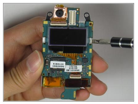
• Prop out the LCD screen using a Small Flathead Screwdriver.
