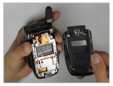
• Completely remove the outer casing from the phone.
