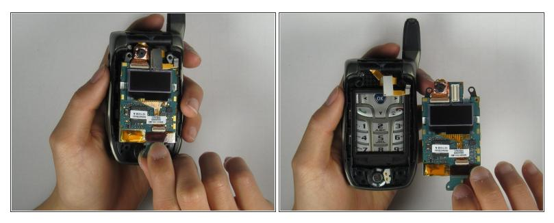
• Remove the LCD board from the phone by grabbing the bottom side of the LCD board.
