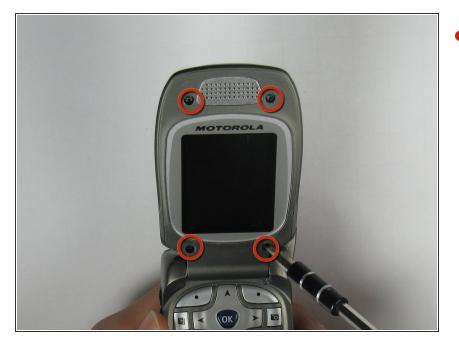
Unscrew the screws using a Phillips #00 Screwdriver.
