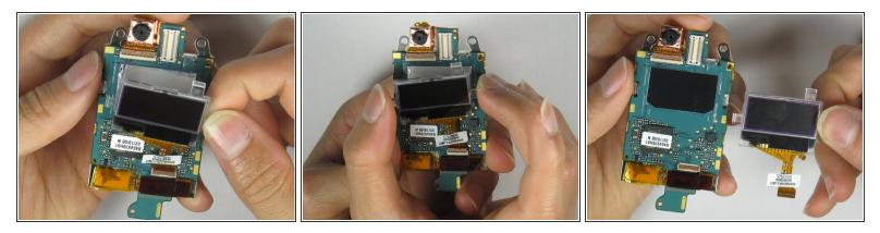
• Remove the LCD screen from the LCD board.
