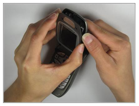
• Gently separate the flip cover case from the phone with your hands when the crack is wide enough.
