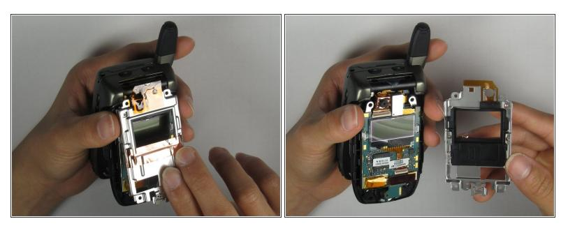
• Place your thumb underneath the protective metal covering to remove it from the phone.
